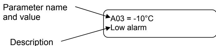
Use the up/down keys to scroll the various parameters.
